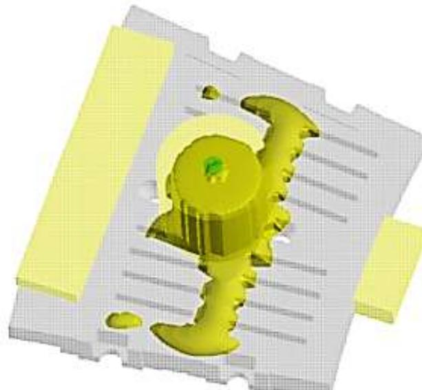
Fig. 2. The disrupted supply flow of the diaphragm casting design simulation in the previous research
